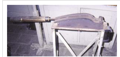
Bending iron for the sides of the bandura
