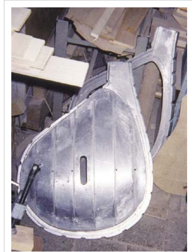
Aluminum mould for the gluing of the backs of the bandura
